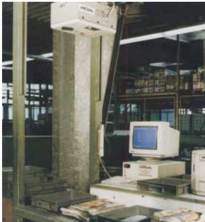
Due to its scanning depth of 80 cm, the scanner can reliably read bar codes displayed on magazine bundles of various height.
